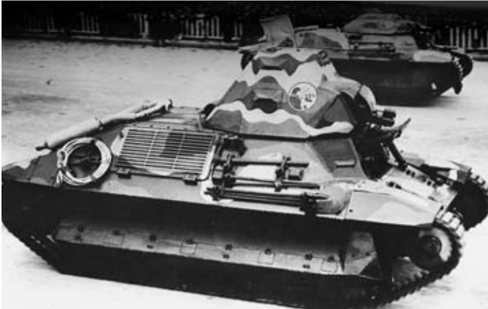
French FCM-1936 light tank. While possessing effective armor protection for the era, it had only a one-man turret and carried no radio.
