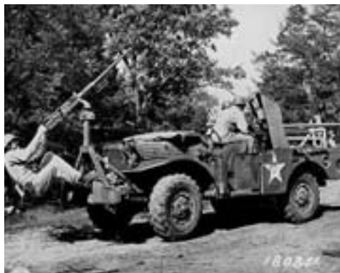
M6 Gun Motor Carriage modified through the addition of an awkwardly mounted anti-aircraft machine gun
