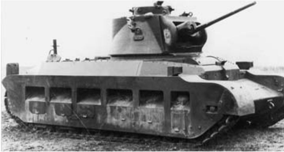
1937 prototype of the Matilda II, one of the most heavily armored tanks at the start of World War II
