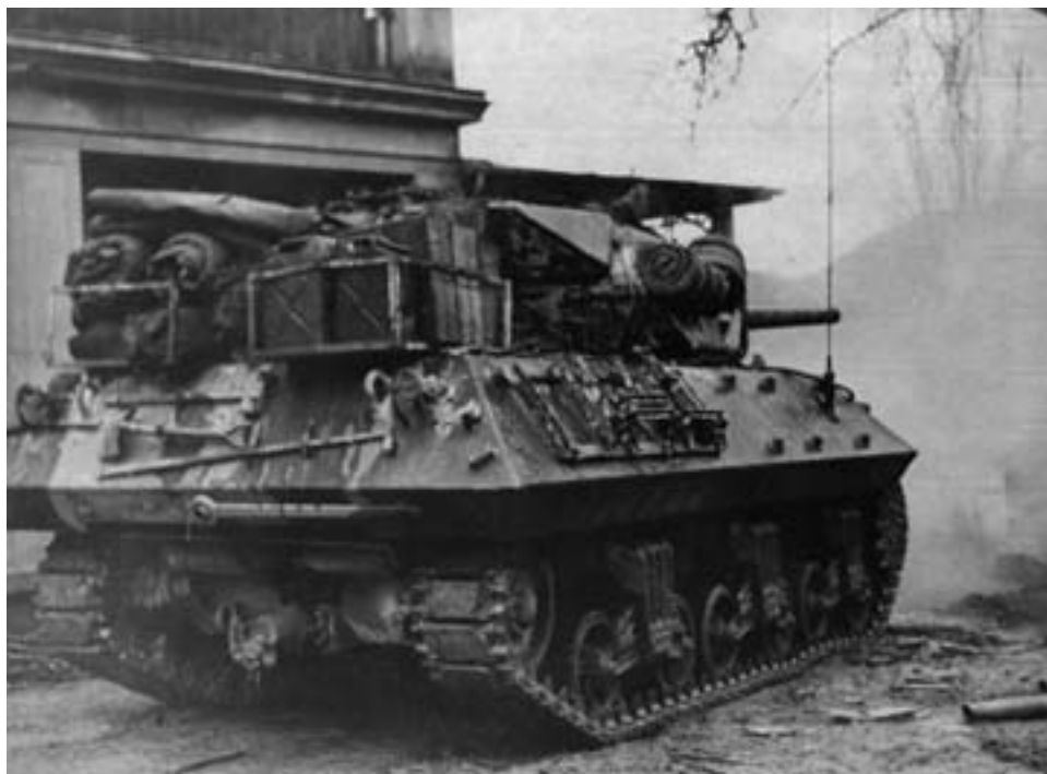
M10 Gun Motor Carriage loaded with personal gear, tenting, and extra gasoline for sustained operations in the field
